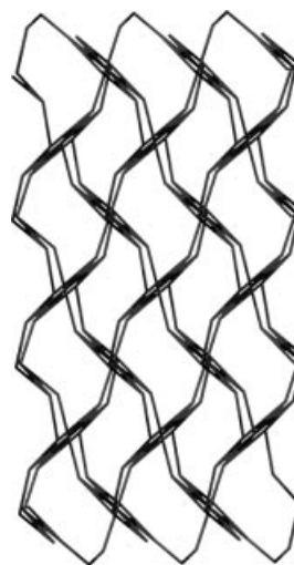
Figure 4. View of the noninterpenetrating decorated rutile net with the (4.6^2)_2(4^2.6^{10}.8^3) topology and constructed from distorted octahedral Co 3 SBUs and triangle BTC 3- units.
